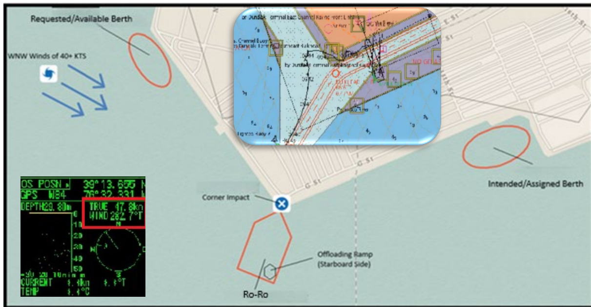
Figure 2: Facility terminal layout illustrating the allision and grounding with graphic overlays of the vessel's intended track line and wind data.
